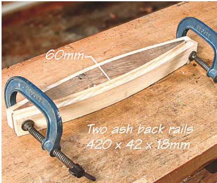
▲ Pic. 4 Here Jeff bends the steamed rails against a former
